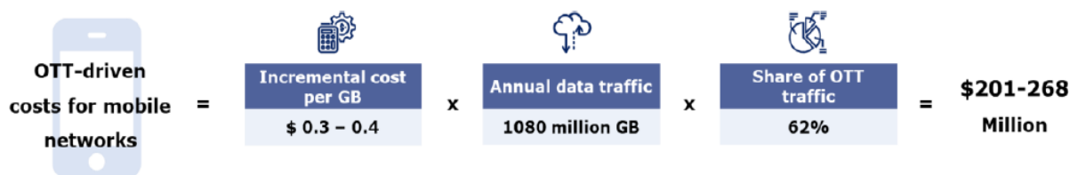
Figure 3: Quantification of the annual OTT-driven costs for mobile networks in the Caribbean region
